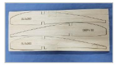
Once again savings on wastage can be made by making a mirror image and putting multiple images to suit the sheet width .--->
